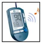
Insert a new test strip into your meter. Place the square end of the strip with the 3 contact bars as far into the meter as it can go. Your meter will greet you and confirm the date and time. It is now ready for use.
